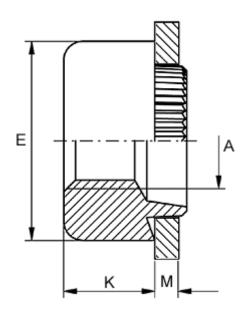
Female thread A = M16Height K = 10.0Outer diameter E = 25.0Plate thickness = 5.0Recommended bore diameter for extreme load = 19.0Recommended bore diameter for normal use = 20.0
